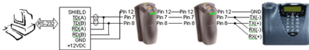
Figure 14: Wiring Diagram for RS-232/RS-485 Converter
