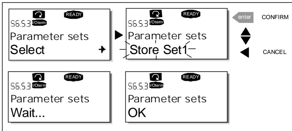
Figure 7-20. Storing and loading of parameter sets
