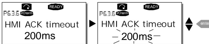
Figure 7-15. HMI acknowledge timeout
