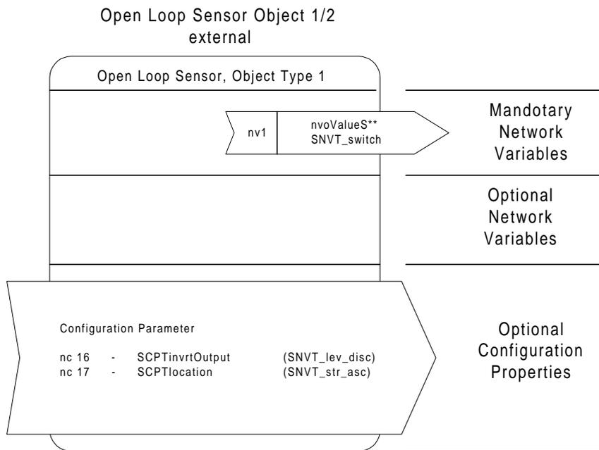
\*\* Timeframe for sending value over LON-Bus adjustable via nciMaxSendTime included in Node Object
