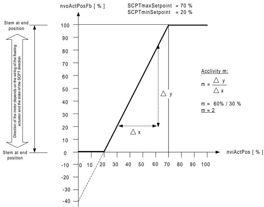
Fig. 16 Diagram# 2 Example for customer adjustment acclivity = 2
