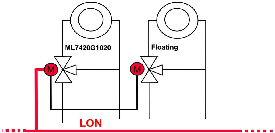
**Fig. 6 Example for ML7420G1020 application**
