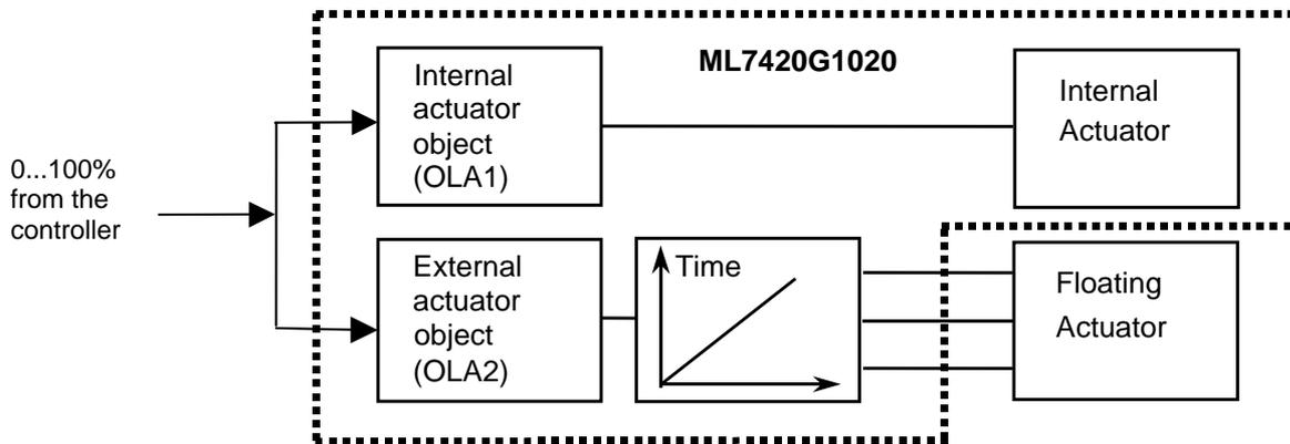
**Fig. 7 Block diagram of ML7420G1020**
