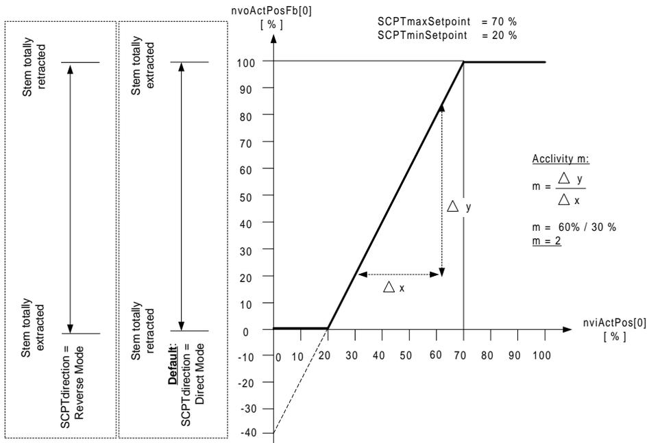
Fig. 12 Diagram# 2, Example for customer adjustment acclivity = 2
