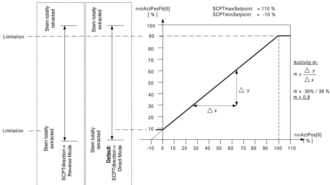
Fig. 13 Diagram# 3, Example for customer adjustment limitation for motor stroke 10%...90%
