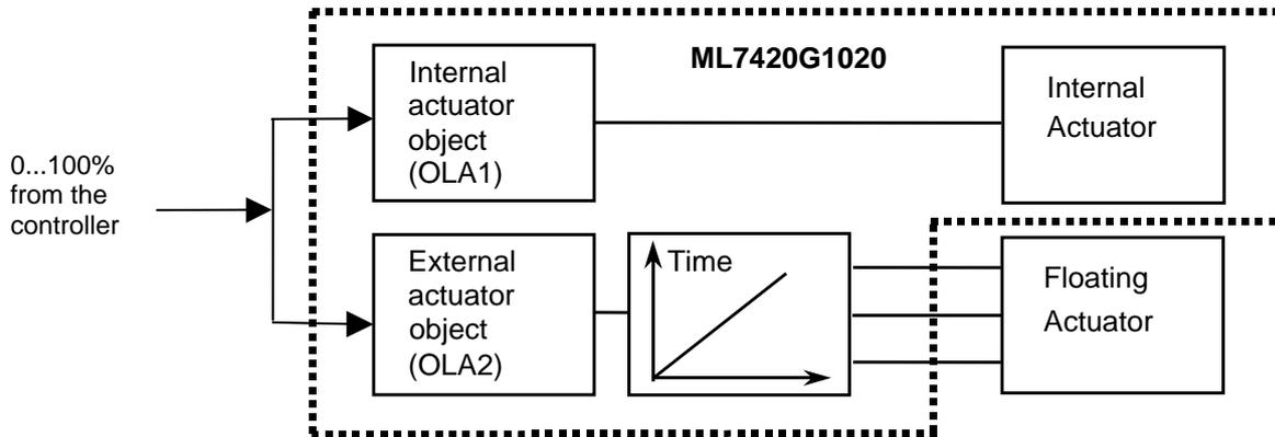
**Fig. 7 Block diagram of ML7420G1020**
