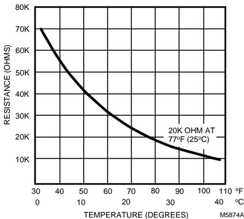
**Fig. 1. Temperature vs. resistance for 20k ohm sensor**
