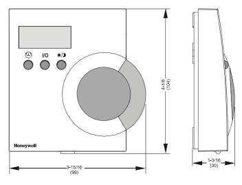
Fig. 6. DWM dimensions in inches (mm)
