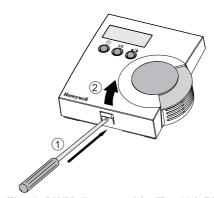
Fig. 1. DWM disassembly (T7560A,B)
