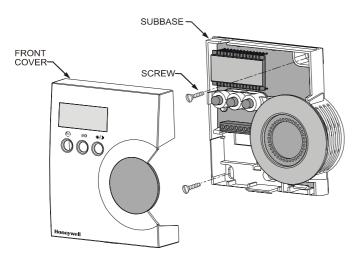
Fig. 3. Mounting of DWM (T7560A,B shown)
