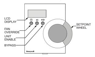
Fig. 7. Control elements of T7560A,B DWM
