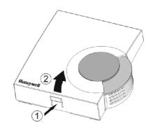
Fig. 2. DWM disassembly (T7560C)
