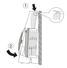
Fig. 5. Mounting cover of T7560A,B DWM.
