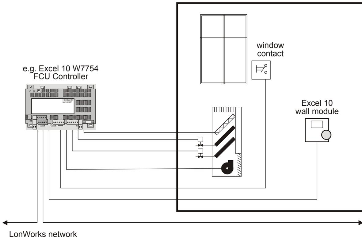
Fig. 2. Typical Fan Coil Unit control application
