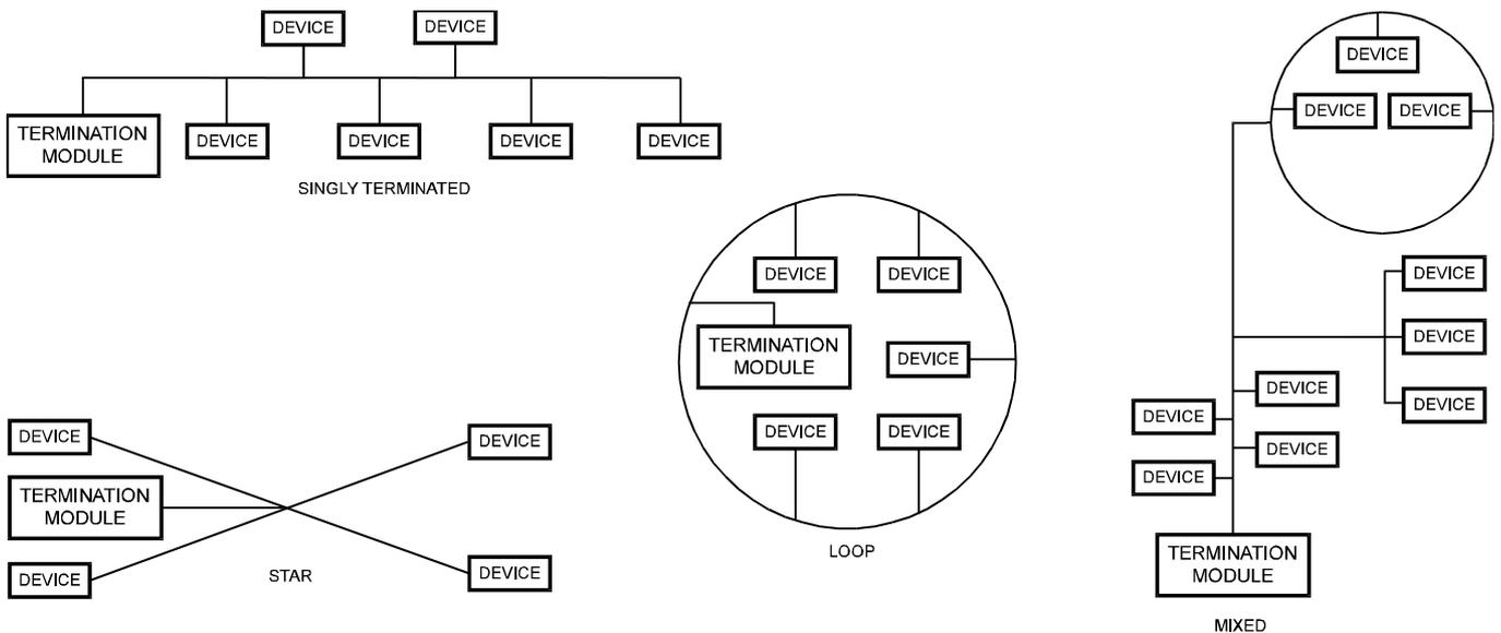
Fig. 15. Free topology LonWorks layout examples
