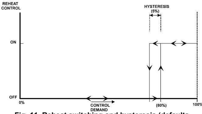
Fig. 11. Reheat switching and hysteresis (defaults shown)
